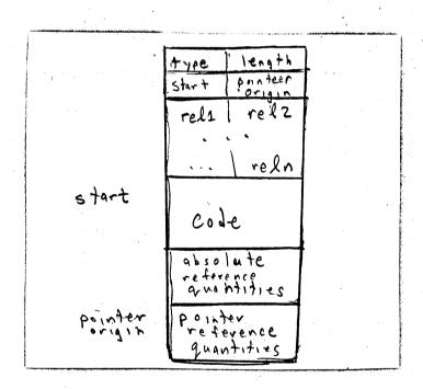
Figure 1: Format of a Compiled Function
