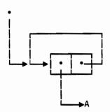
Figure 6. Box representation of a circular list.
