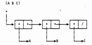
Figure 5. Box representation of list, corresponding to list notation.
